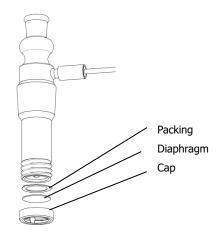
When handling the diaphragm, please use the rubber gloves or tweezers by all means.
