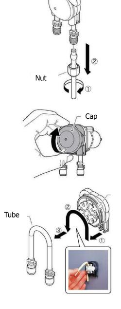
4) Apply the supplied grease around the new tube and axle of cassette.
