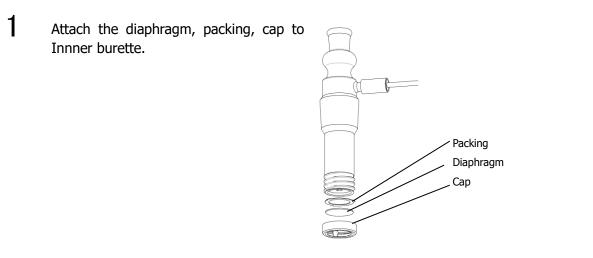
When handling the diaphragm, please use the rubber gloves or tweezers by all means.
