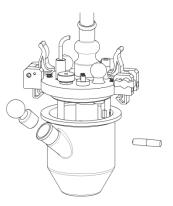
Place the titration cell onto the titration holder, and plug in the cable from the inner burette and the electrode. Tighten the plug screws firmly.
