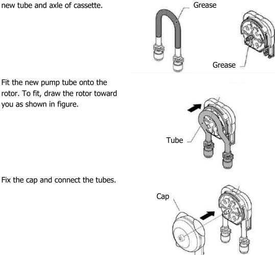
6) Fix the cap and connect the tubes.
