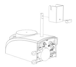
4) Fix the titration cell to the cell holder.
