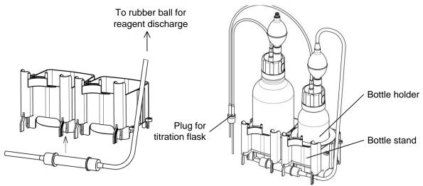
9) Insert the Plug for titration flask carefully into the titration cell. At this point, apply a small amount of KF grease on slide contact area.
