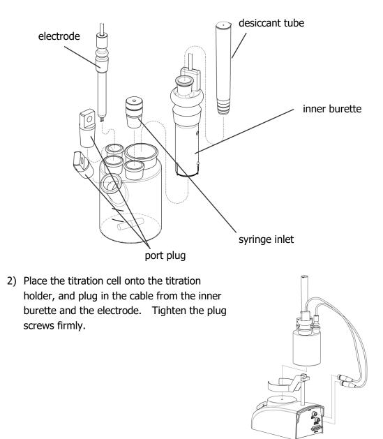
Make sure to apply KF grease around glass sliding area.
