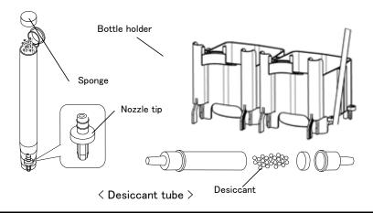
If the nozzle chip slips from the desiccant tube when replacing the desiccant, ensure that you return the nozzle chip in the tube with its trenches downward as shown above.
