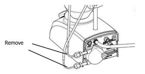
2) Insert the dropping pipette to the tip of the pump tubing or tube, remove the clogging.
