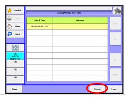
The file selected on USB flash drive will be deleted and the screen display will return to "Loading/Deleting User Table". When deleting further files of sample setting, repeat the above steps 1).
