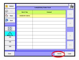
The file selected on USB flash drive will be deleted and the screen display will return to "Loading/Deleting Titration Result". When deleting further files of titration results, repeat the above steps 1).
