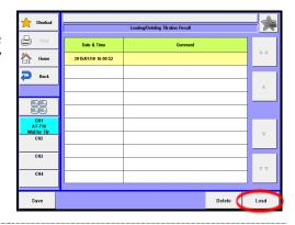
The screen of "Titration Results List (USB Flash Drive)" will be displayed. Then, select the titration result to be displayed on the measuring unit and press [Load] button.
